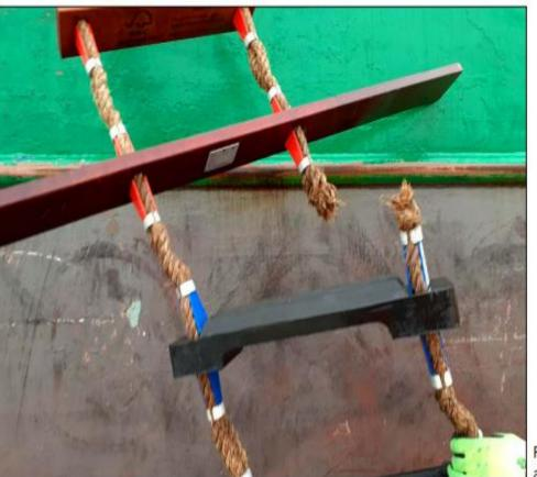
Figure 2: Example of a failed pilot ladder
