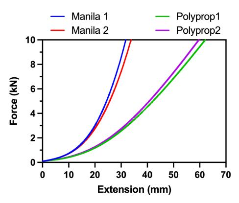
Stress-strain graph (force-extension) of the behaviour of the Manila and Polyprop ropes under test during run 10.
