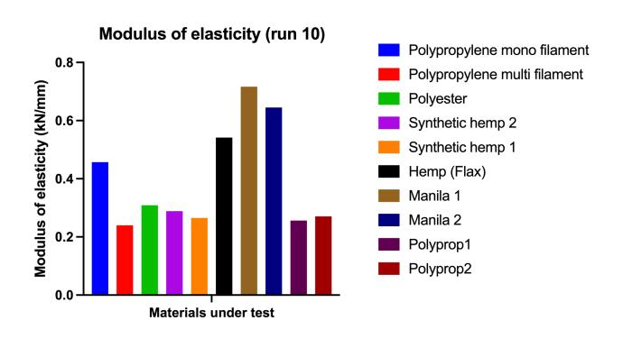
Stiffness data (modulus of elasticity) recorded during run 10 (linear section of data when force > 6kN).
