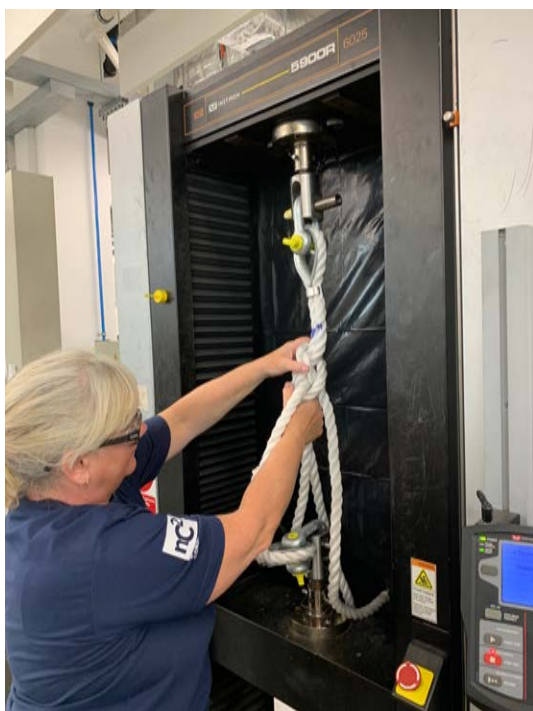
Figure 32: Slip and Grip Scenario 1 being tested on the Instron 6025 electromechanical testing machine.
