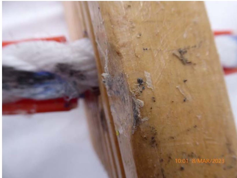
Figure 67 : Specimen N after 1500 cycles showing the damage that the large shackle did to the wooden step.
