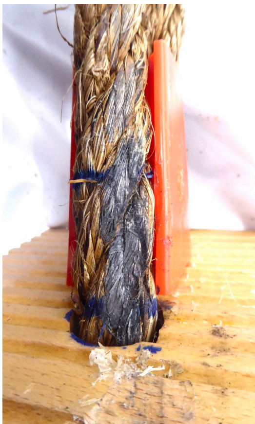
F: Maninla rope (manila seizing) large shackle. G: Maninla rope (metal clip) large shackle
