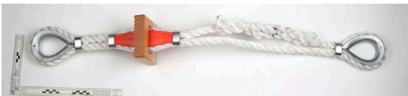
K: 20 mm polypropylene rope, with step and metal clip seizing (sample L the same)
