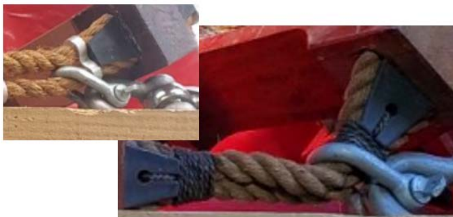
Figure 5: An example of 'D' shackles being used as a tie-off method.
