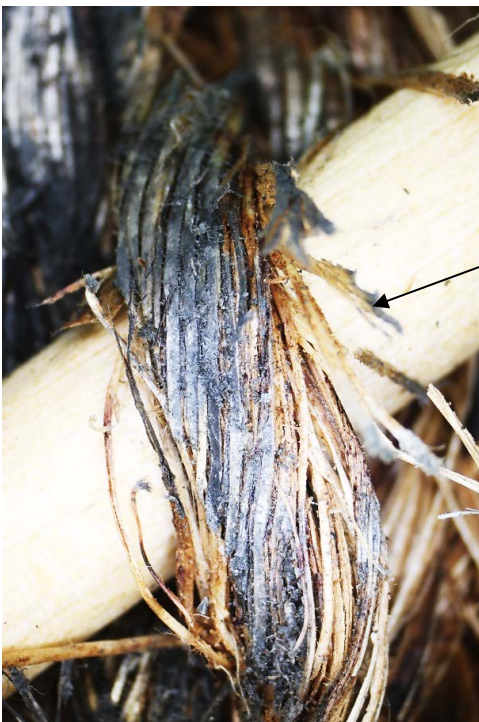
Figure 75 : Macroscopic images of the worst worn strands from Manilla and the Polypropylene rope material.
