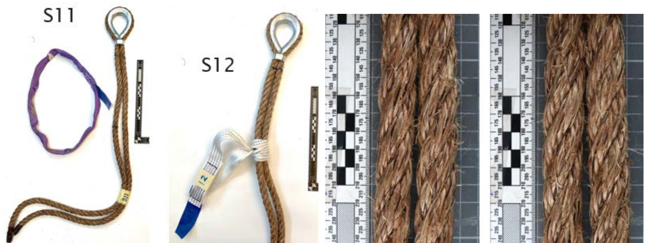
Figure 54: Scenarios 11 and 12 post-test (Left) and the examined worn section of the double rope (Right).
