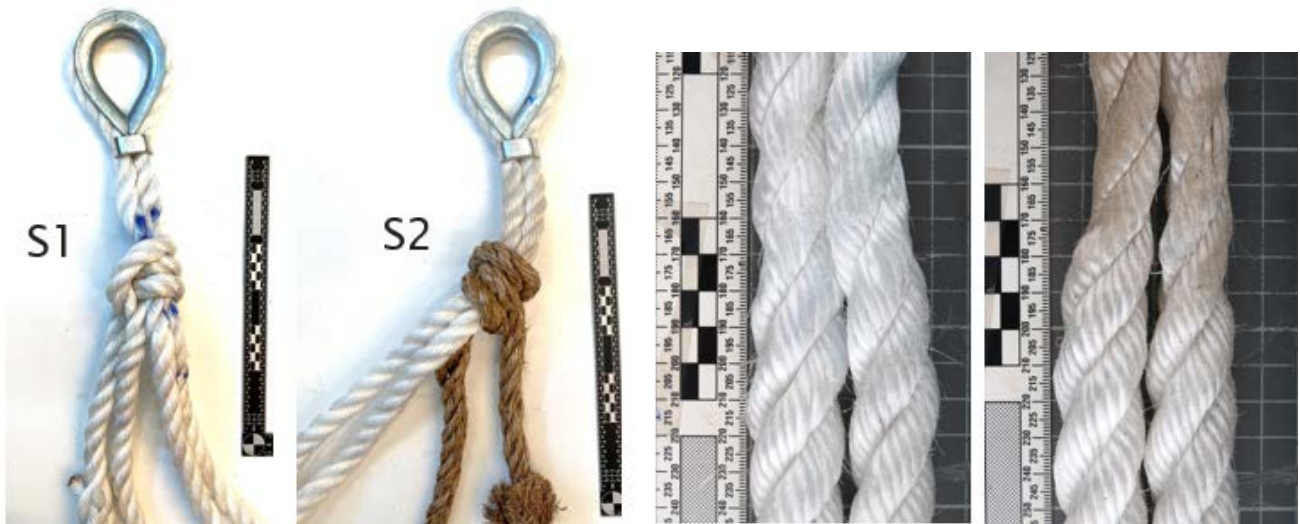
Figure 49: Scenarios 1 and 2 post-test (Left) and the examined worn section of the double rope (Right).
