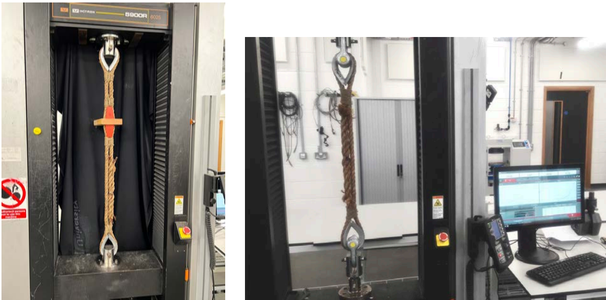
Figure 11: Tested in tension on an Instron 6023 Electromechanical test machine, operating with Instron Bluehill Universal software and fitted with a 100 kN load cell.
