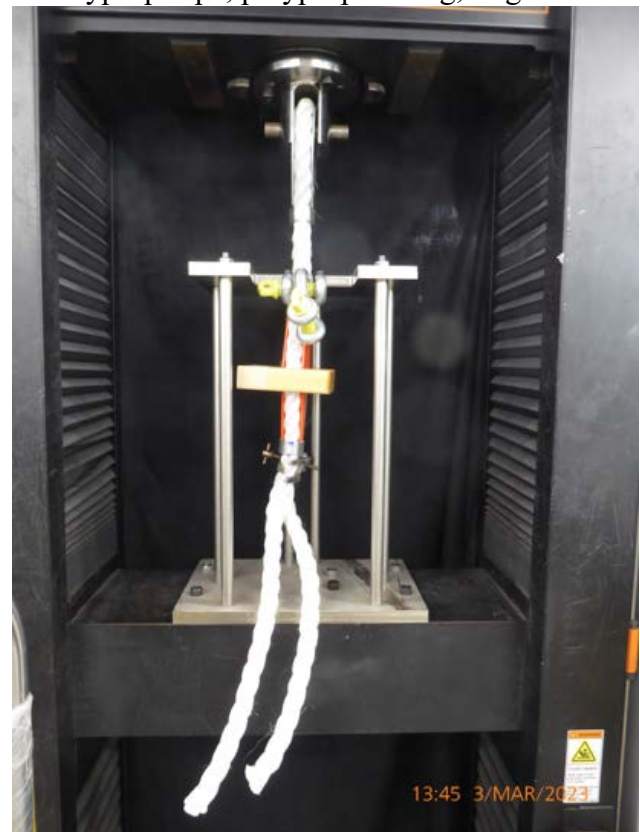
P: Polyprop rope, metal clip, small shackles
