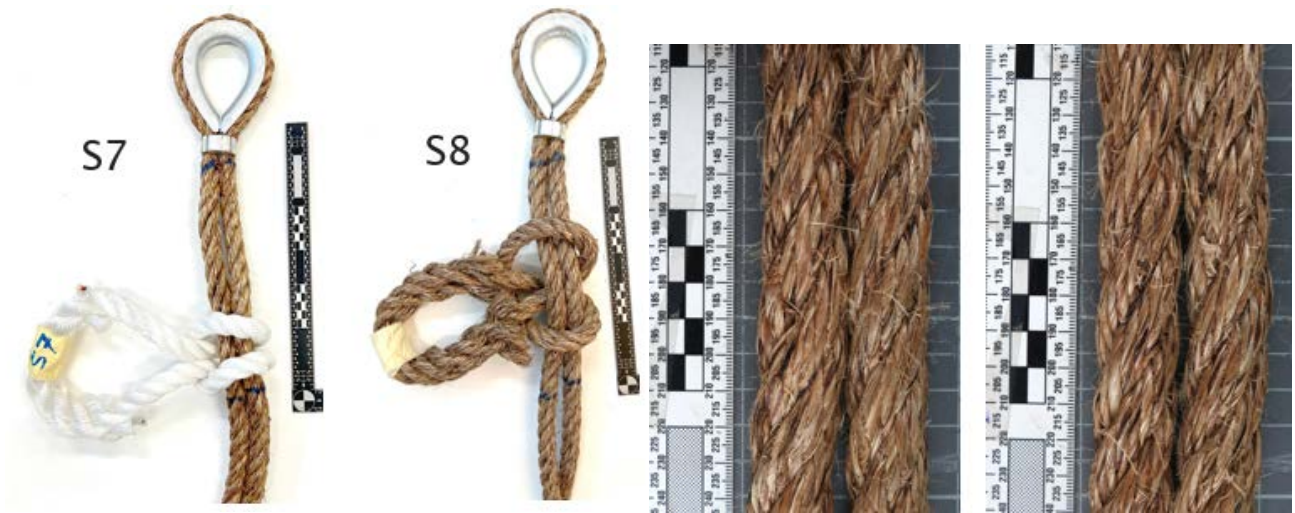
Figure 52: Scenarios 7 and 8 post-test (Left) and the examined worn section of the double rope (Right).
