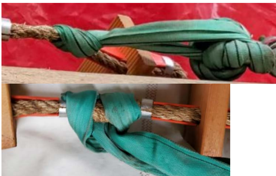
Figure 6: An example of loading straps (cargo lifting devices) being used as a tie-off method.
