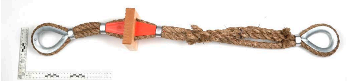
C: 20 mm manila rope, with step and metal clip seizing (sample D the same)
