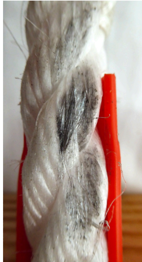
E: Manila rope (manila seizing) small shackle. M: Polyprop rope (polyprop seizing) small shackle.
