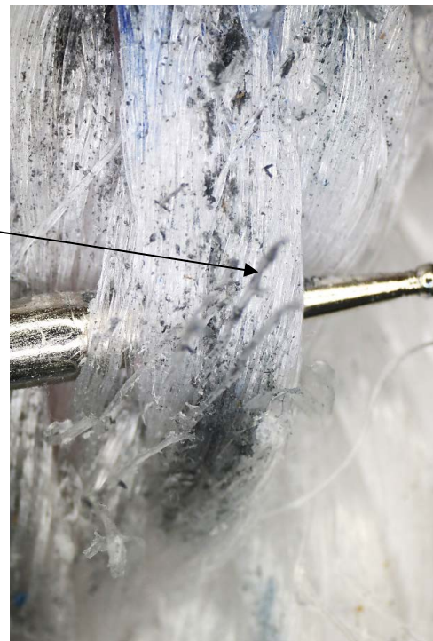
Figure 75 : Macroscopic images of the worst worn strands from Manilla and the Polypropylene rope material.
