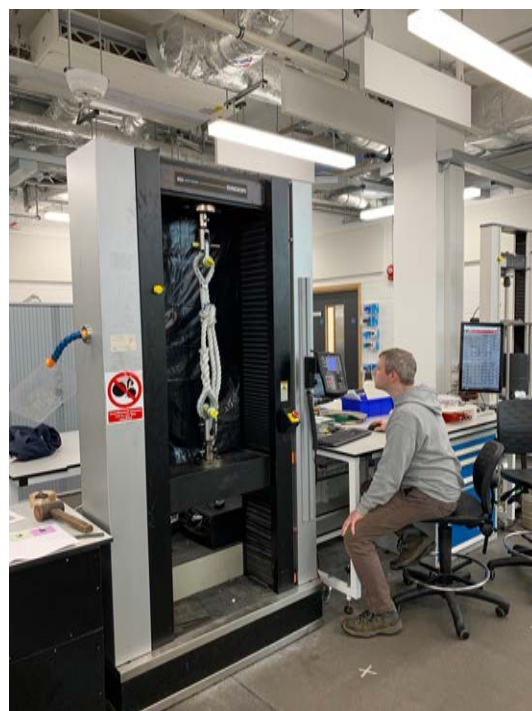
Figure 32: Slip and Grip Scenario 1 being tested on the Instron 6025 electromechanical testing machine.
