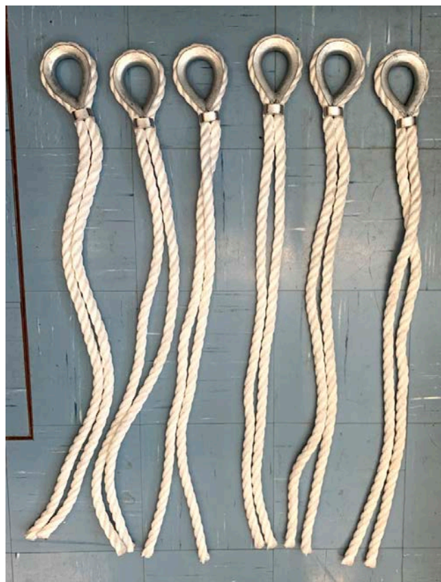
Figure 30: Examples of the polypropylene rope pairs provided for WP2 (manila pairs also provided).
