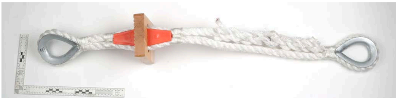
I: 20 mm polypropylene rope, with step and polypropylene seizing (sample J the same)
