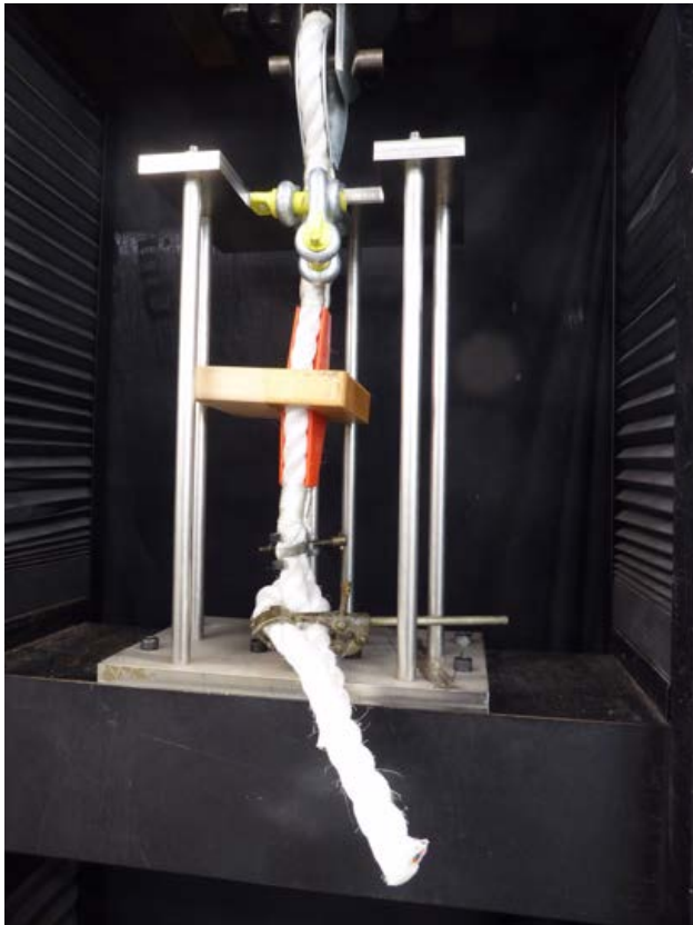
M: Polyprop rope, polyprop seizing, small shackles N: Polyprop rope, polyprop seizing, large shackles
