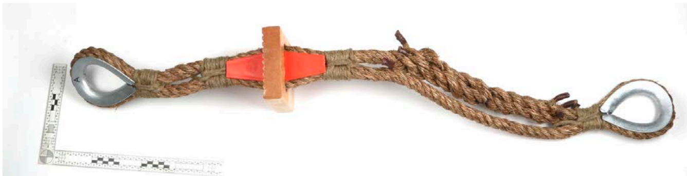
A: 20 mm manila rope, with step and manila rope seizing (sample B the same)
