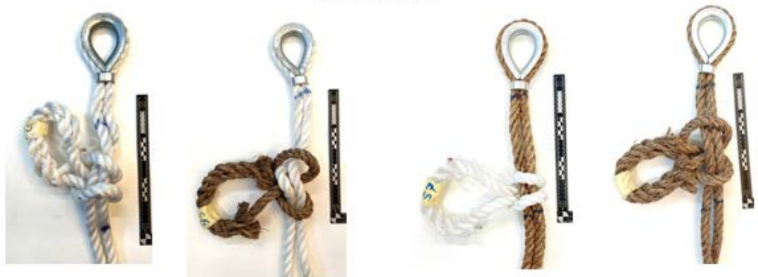
Figure 46: Max force for cow hitch scenarios involving polypropylene and manilla loops.
