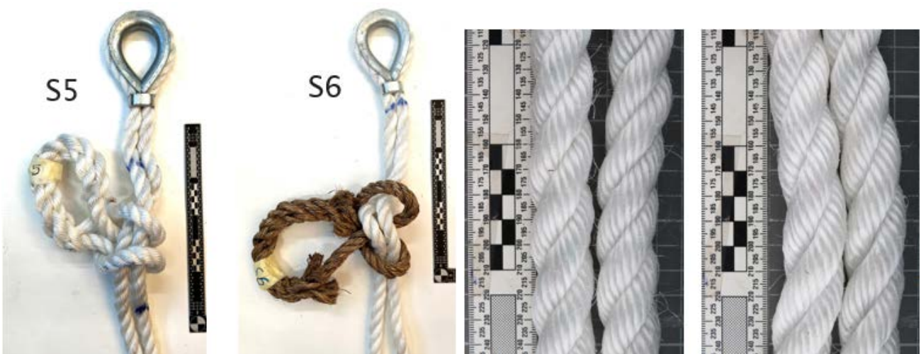
Figure 51: Scenarios 5 and 6 post-test (Left) and the examined worn section of the double rope (Right).
