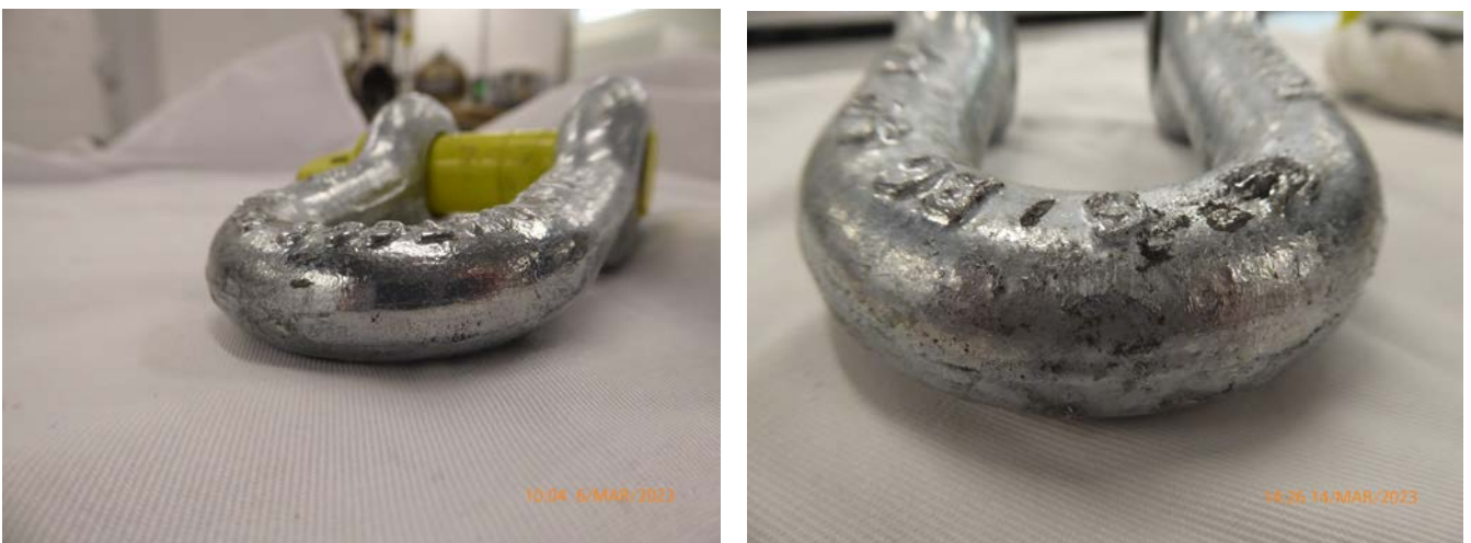
Figure 64 : No visible damage was found on the shackle after any of the tests.
