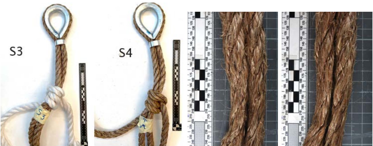
Figure 50: Scenarios 3 and 4 post-test (Left) and the examined worn section of the double rope (Right).
