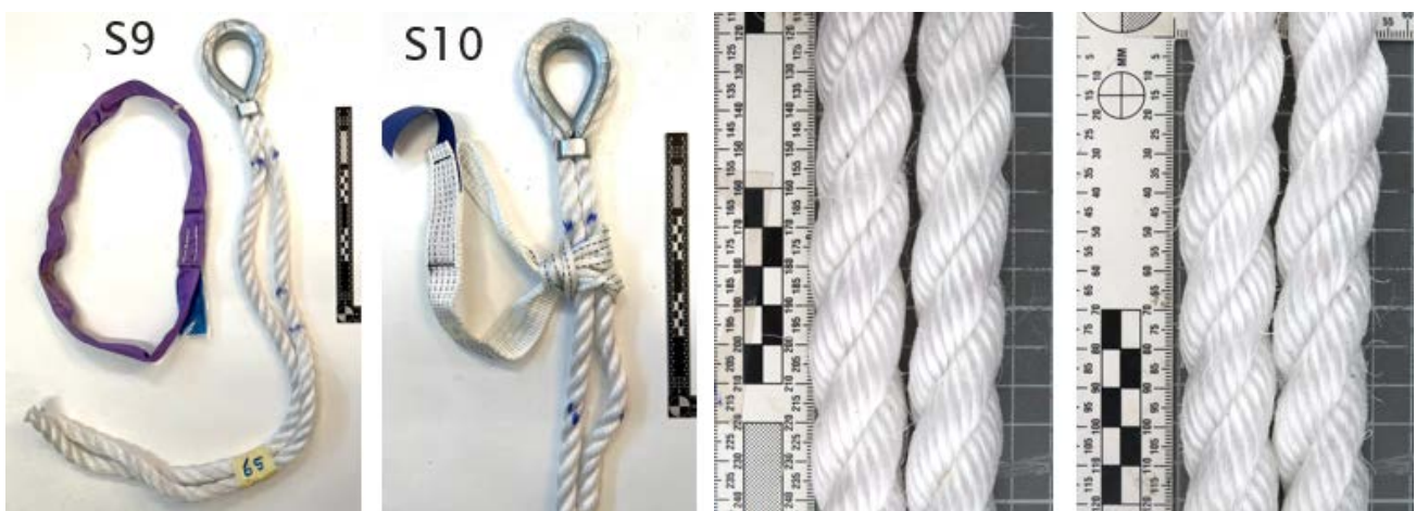
Figure 53: Scenarios 9 and 10 post-test (Left) and the examined worn section of the double rope (Right).
