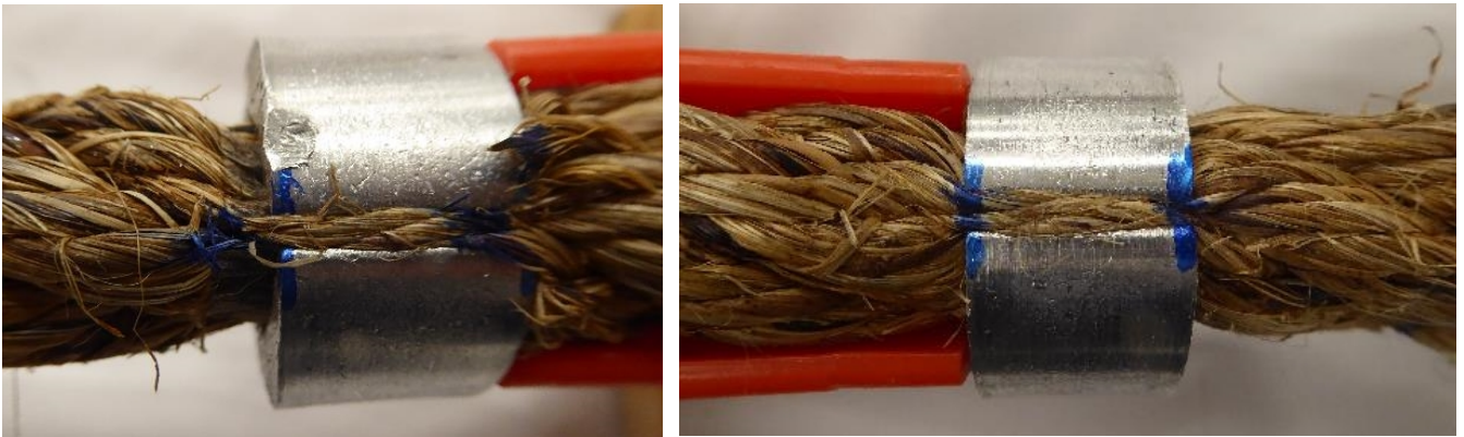
Figure 63 : Specimen H after 1500 cycles showing (Left) permanent plastic deformation to the top of the metal fastener from contact with the small shackle. The top metal fastener slipped 2 – 3 mm from its initial position during the test. (Right) No slippage was observed on the metal fastener underneath the wooden assembly.
